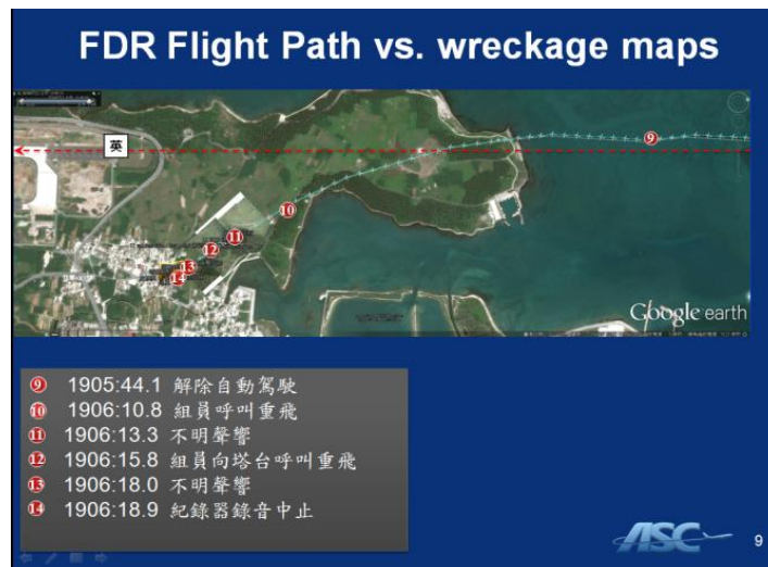
Fig.1 The FDR (ATR's flight data recorder) flight path versus wreckage map during the last 34 seconds for TransAsia Airways GE222 Occurrence at Makung Airport in Penghu Island on 23 July 2014 based on the Aviation Occurrence Report prepared by Aviation Safety Council in 2016.
